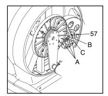
of the elliptical exerciser until the Belt (57) is tight. Then, tighten the three screws.
